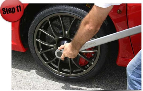
While off the ground, with an assistant holding the brake pedal down firmly, tighten the wheel nut in the correct direction, to 300 Nm or 220 ft.-lbs
