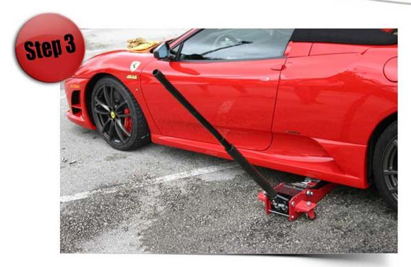
Raise the vehicle on one side and slide jack stands under the frame. Remove the wheels carefully and do not 'bump' against the brake discs.
