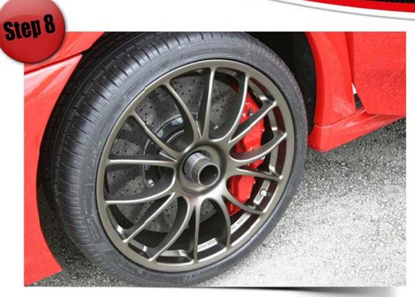
Carefully slide your wheel over the new center lock adaptor. <u>Take care to not bump the wheel against the brake caliper and brake-disc or rotor.</u>
