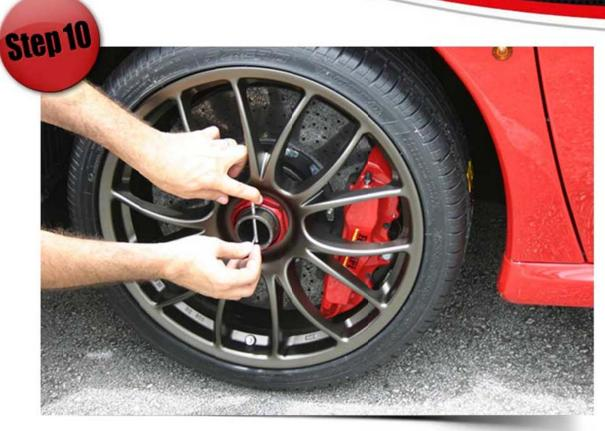
Slide the safety lock-pin into place as shown.
