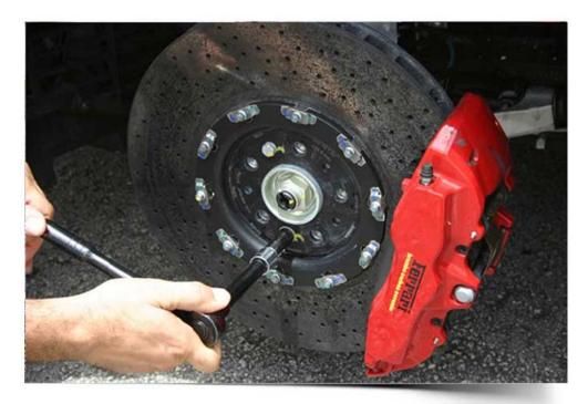
Avoid moving the brake disc assembly at this time so as not to misalign the bolt holes. Make sure that the flat surfaces are clean from grit and road dirt.
