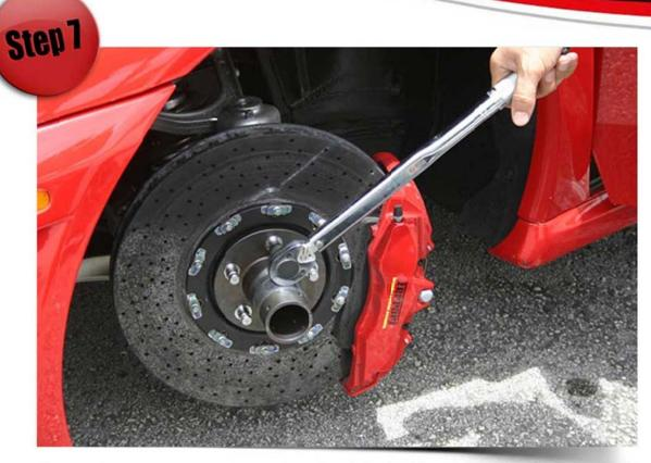
Using a torque wrench and a six sided 13mm socket, tighten the bolts to 130 Nm or 96 ft.-lbs. Always tighten the bolts in a criss-cross pattern.
