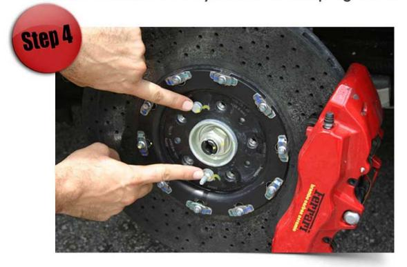
Remove the two fasteners as indicated. The bolt head is a 13mm and the pin-head is a 12mm.
