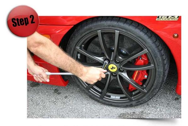
Loosen the wheel bolts slightly to facilitate removal when the wheels are of the ground. Do not over loosen the bolts.
