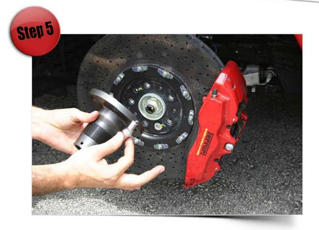
At this stage, make sure that you have an adaptor with <u>Right Hand</u> thread for the Left side of the car and an adaptor with <u>Left Hand</u> thread for the Right side of the car.
