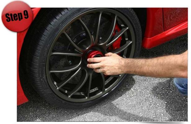
Fit the center-lock nut over the stub and hand-tight it.
